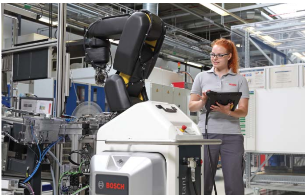
The APAS mobile production robot works closely with human colleagues, without coming into physical contact with them.
